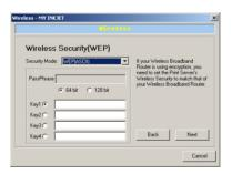
**64-bit WEP** - To create a set of 64-bit WEP ASCII keys, activate one or more keys by clicking in the appropriate circles, then enter five standard characters (numbers or letters) in each activated **Key** text box (**Key 1-**, **Key 2-**, **Key 3-**, **Key 4-**). After activating 64-bit WEP on the Print Server, a computer with wireless capability can use the Print Sever only if these same keys are entered in the computer's wireless encryption scheme.
